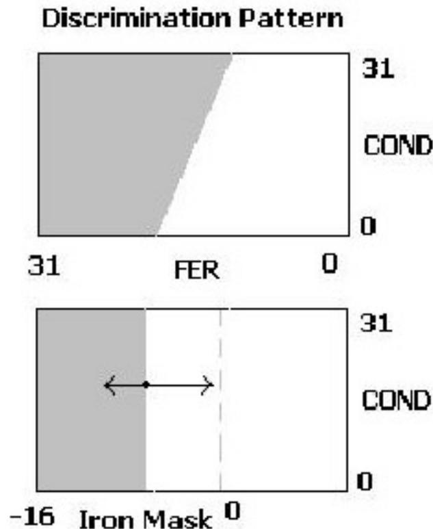
**All Metal** - is the term used to describe a clear discrimination pattern - that is accepting ALL targets whether ferrous or non-ferrous. To select All Metal press the shift button next to the AM icon to reduce Iron Mask and clear the discrimination pattern. Bear in mind that A.M. might be "noisy" on certain soils that might have high levels of mineralization in them.
